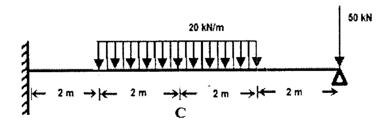
3. Draw Shear force and bending moment diagrams for the fixed beam shown in fig.
