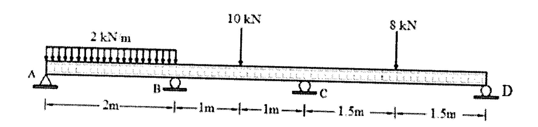
5. A continuous beam is as shown in fig. the support D sinks by an amount of 5/EI. Analyse the beam by using slope deflection method?
