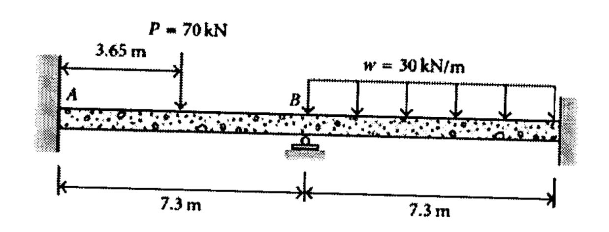
4. Analyse the continuous beam shown in fig. by using Clapeyron's theorem of three moments.
